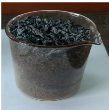
Fig. 1: Tree-like structure (dendritic structure) of barium hexaferrite after auto-combustion and before any annealing treatment.
